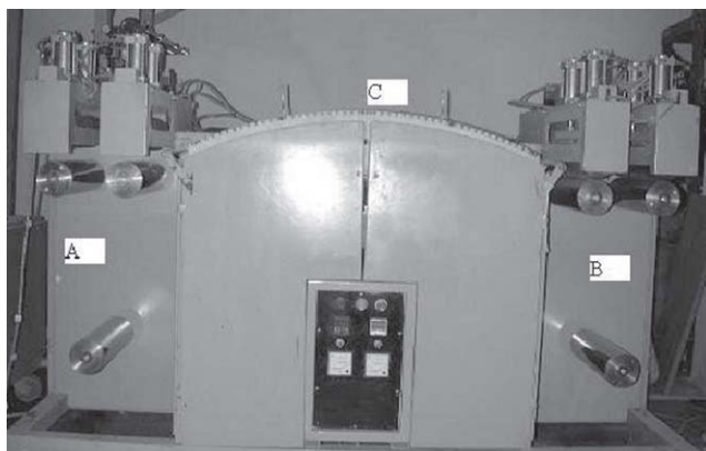
Figure 2 Continuous stretching unit (A) Godet 1, (B) Godet 2, and (C) Hot plate.
